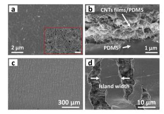
Fig. 2 SEM results of the fabrication process. (a) Top view SEM image of the CNTs films/PDMS composite. Inset: Top view SEM image of multilayer CNTs films, scale bar: 1  $\mu m$ . (b) Cross-sectional SEM image of the CNTs films/PDMS strain sensor, showing the top conductive layer (CNTs films/PDMS) and bottom elastic layer (PDMS). (c) SEM image showing the network cracks, reflecting the homogeneous fracturing of CNTs films/PDMS composite. (d) The arrows indicating the island width.
