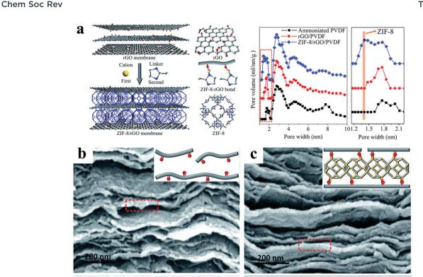
Fig. 8 Microenvironments of 3D nanochannels and bulk structures in 3D(MOF)/2D membranes. (a) Schematic diagram of 3D nanochannels in ZIF-8/rGO membranes (left), pore size distributions of the ammoniated PVDF hollow fiber, rGO membrane and ZIF-8/rGO membrane (right). (b and c) Cross-sectional images of rGO and ZIF-8/rGO membranes. Reproduced with permission from ref. 39. Copyright 2016, Royal Society of Chemistry.
