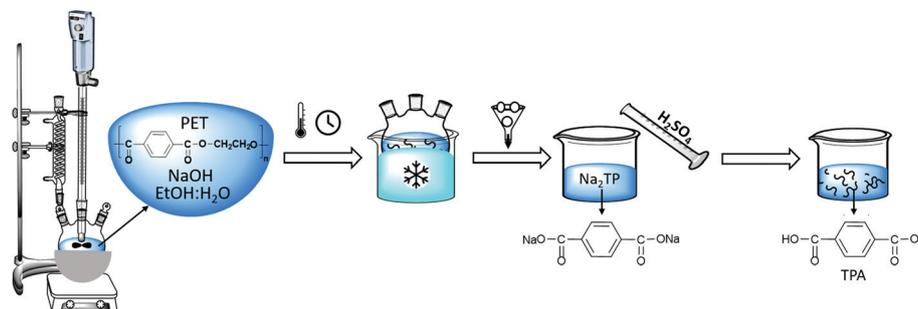
**Scheme 2** Experimental set-up of PET alkaline hydrolysis.
