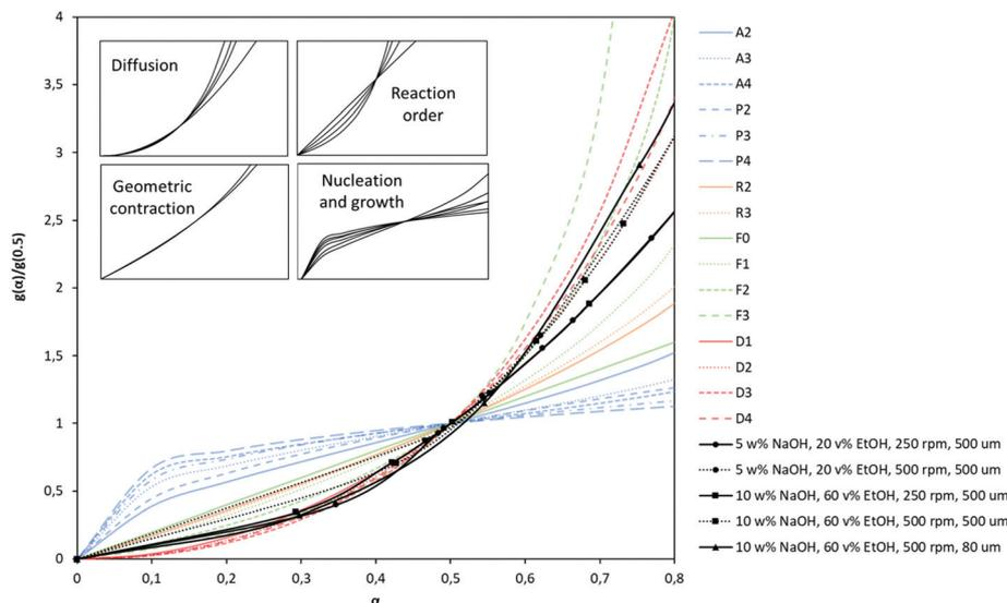
**Fig. 3** Theoretical kinetic master curves plotted as integral form of reaction models at isothermal condition ( $g(\alpha)/g(0.5)$ ) versus conversion fraction ( $\alpha$ ) and superimposition of experimental kinetic data on these kinetic models ( $R^2$  values and best-fit diffusion kinetic models can be found in Appendix, Table A-1 and Fig. A-3).
