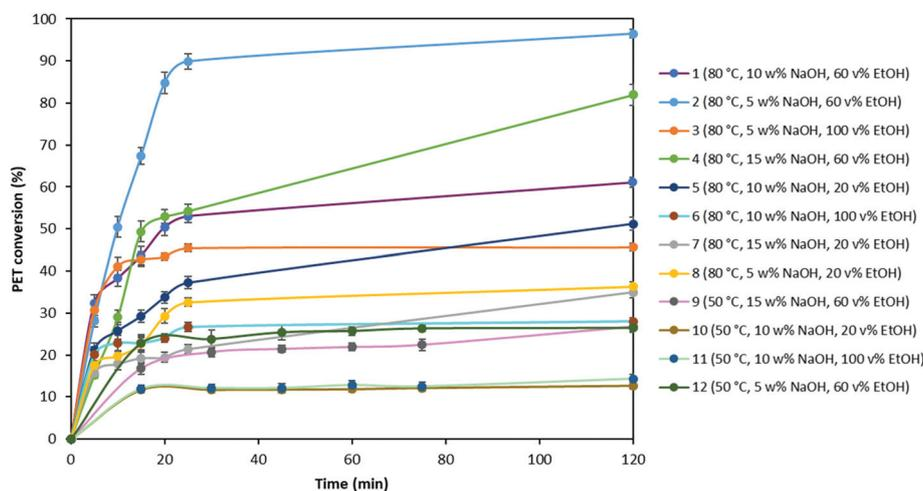
Fig. 2 PET conversion at different experimental conditions (0.02 g mL<sup>-1</sup> PET flake with 500 μm particle size, stirring at 250 rpm with a magnetic stirrer).
