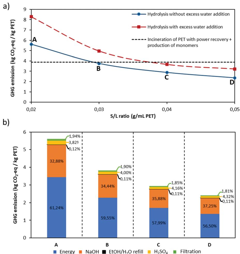
**Fig. 7** (a) GHG emission of PET alkaline hydrolysis (kg CO<sub>2</sub>-eq per kg PET) with and without excess water addition at different S/L ratios (g mL<sup>-1</sup> PET) and comparison with GHG emission of incineration of PET with energy recovery together with production of equivalent amount of PET monomers; (b) contribution of different steps/inputs to the total GHG emission of the PET hydrolysis process without excess water addition (%) at each S/L ratio.
