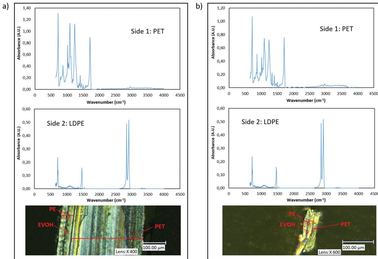
Fig. 1 (a) FTIR spectra of both sides of multilayer PET tray and its POM image (b) FTIR spectra of both sides of multilayer PET film and its POM image.
