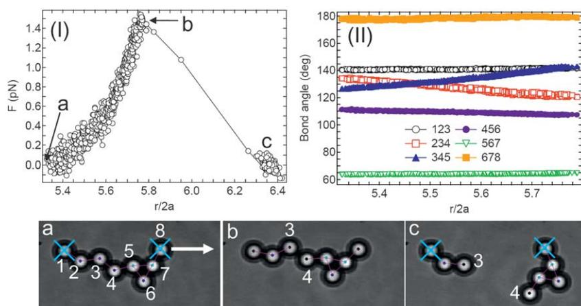
**Fig. 2** (I) Force profile and (II) bond angle change during the applications of tension to a small aggregate formed with 25  $\mu\text{M}$  SPAN 80 in the decane super-phase (SP1). The bottom images (a-c) show snapshots corresponding to the moment of discontinuity in the force profile. The colors on the particles correspond to their bond number.
