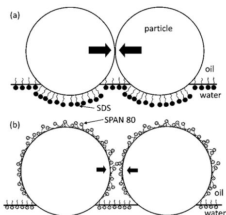
**Fig. 4** Proposed origin of the difference of aggregate rigidities under the conditions of SDS in the sub-phase (a) and SPAN 80 in the super-phase (b). The particle at the interface in both conditions dominantly belongs to the oil-side, compared to the one at the neat oil–water interface (*i.e.*, neutral wetting).<sup>34</sup> SPAN 80 molecules adsorbed in the super-phase on the particle surface, considering the relatively polar alcohol head groups. The scale is exaggerated for illustration.
