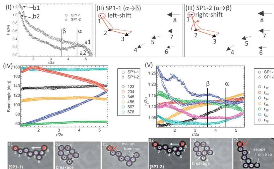
**Fig. 3** Micromechanics of aggregate during the first (SP1-1) and second (SP1-2) compressions. This aggregate is reformed from the ruptured aggregate (SP1) in Fig. 2. Force profiles (I), movement vectors (II, III), bond angle changes (IV), and particle separations between two neighboring particles (V). The bottom images are the corresponding aggregate images. The colors on the particles correspond to their bond number.
