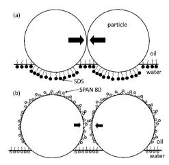
**Fig. 4** Proposed origin of the difference of aggregate rigidities under the conditions of SDS in the sub-phase (a) and SPAN 80 in the super-phase (b). The particle at the interface in both conditions dominantly belongs to the oil-side, compared to the one at the neat oil—water interface (*i.e.*, neutral wetting).<sup>34</sup> SPAN 80 molecules adsorbed in the super-phase on the particle surface, considering the relatively polar alcohol head groups. The scale is exaggerated for illustration.
