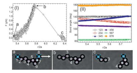
Fig. 2 (I) Force profile and (II) bond angle change during the applications of tension to a small aggregate formed with 25 μM SPAN 80 in the decane super-phase (SP1). The bottom images (a-c) show snapshots corresponding to the moment of discontinuity in the force profile. The colors on the particles correspond to their bond number.
