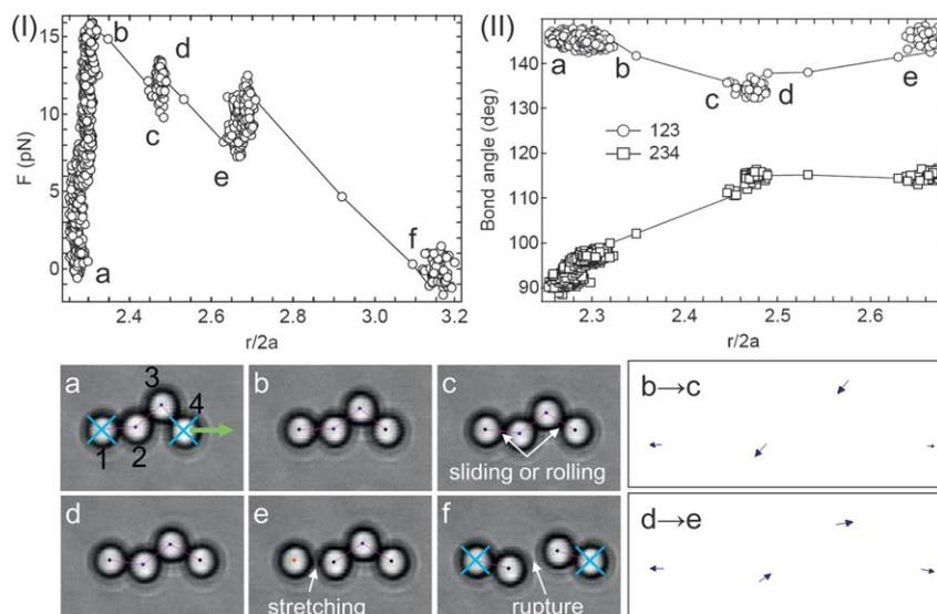
**Fig. 1** Micromechanics of aggregate (SS1) at an oil-water interface containing 0.25 M NaCl and 0.1 mM SDS in the aqueous sub-phase. (I) The force profile during the application of a tensile force with two optical traps and (II) the corresponding bond angle change. In the bottom are image frames corresponding to discontinuities in the force profile. The movement vectors for the steps  $b \rightarrow c$  and  $d \rightarrow e$  are shown to the right.
