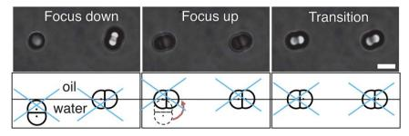
Fig. 3 Transition method for the doublet particles using optical tweezers (see the text). A movie is available in the Supplementary Information†. The scale bar is 5 µm.
