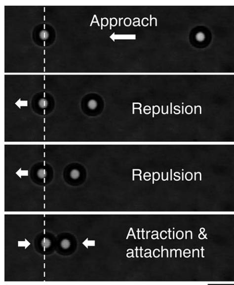
**Fig. 2** Snapshots for the direct measurement of the interaction force between two spherical particles using time-shared optical traps. The left particle is held by a stationary trap while the right particle approaches stepwise by translating its trap. The vertical line indicates the equilibrium position of the particle in the stationary trap. The scale bar is 5  $\mu\text{m}$ .
