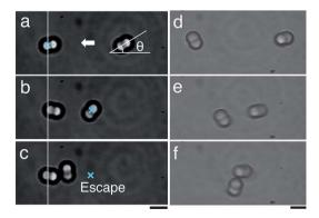
Fig. 7 Snapshots of the force measurements using active (a-c) and passive methods (d-f). The movies of both methods can be viewed in the Supplementary Information.† The scale bar is 5 μm.
