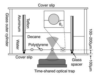
Fig. 1 Schematic of the flow cell.
