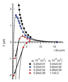
Fig. 5 Four representative force curves from Fig. 4a fitted with eqn (3), (1) and (2). The fitting parameters  $a_2$  and  $a_3$  for each curve are given in the legend. The arrows indicate the jump-into contact due to the mechanical instability when the gradient of the attractive force exceeds the optical trap stiffness,  $\kappa_t$ .
