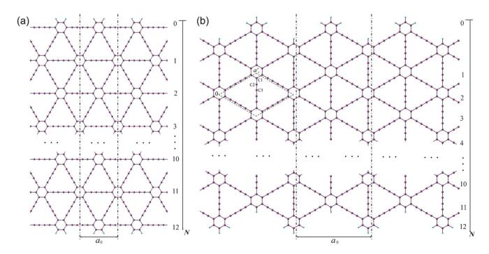
Fig. 1 Models of the 1D graphdiyne nanoribbons with (a): armchair edges (A-NRs); (b) zigzag edges (Z-NRs). The unit cell of the 2D graphdiyne is labeled with the dashed rhombus in Fig. 1(b),  $a_0$  and  $a'_0$  are the lattice constants of the 1D NRs and 2D graphdiyne, respectively.
