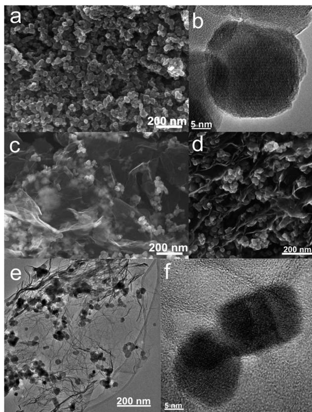
**Fig. 4** (a) SEM and (b) HRTEM images of commercial Fe<sub>3</sub>O<sub>4</sub> nanoparticles; and (c, d) SEM, (e) TEM, and (f) HRTEM images of M2-GNS.
