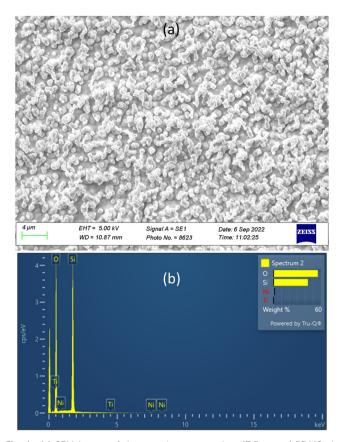
Fig. 4 (a) SEM image of the sample grown using 47.5 mg of PDMS via configuration three, as shown in Fig. 3c. The coating displays island-type growth, characteristic of SiO2 on Si using PVD, with individual islands of  $\sim$  1  $\mu$ m in size, alongside multi-island structures. (b) EDX spectra of the same sample imaged in (a) showing the weight percentages of Si and O signals.
