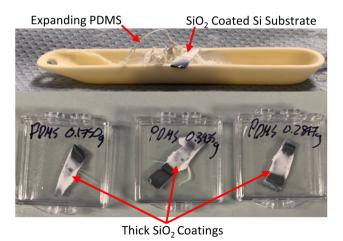
Fig. 2 Photograph of SiO<sub>2</sub> deposition following the procedure of Hu et al., 27 i.e. configuration one, showing the thick coatings and expansion of PDMS during heating.
