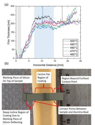
Fig. 8 (a) Steady-state deposition temperature dependence of SiO<sub>2</sub> coating using 6 mg PDMS at a heating rate of 12 °C minute<sup>-1</sup> using updated sample preparation. (b) Annotated top-down photograph of SiO<sub>2</sub> PVD sample highlighting the different coating regions observed in (a).
