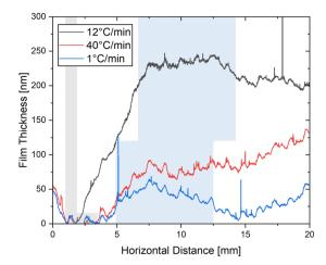
Fig. 10 SiO<sub>2</sub> thickness dependence on heat rate for a steady-state deposition temperature of 500 °C using 6 mg of PDMS.
