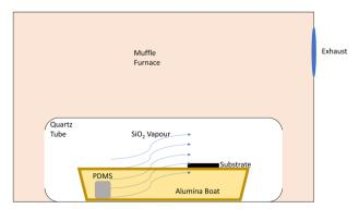
Fig. 1 Schematic diagram of novel PVD system for SiO2 deposition on solid substrates. The substrate is placed between the heated block of PDMS and the exhaust of the muffle furnace, utilising the difference in temperature to drive the SiO<sub>2</sub> vapour over the substrate. The quartz tube ensures most of the vapour is directed over the substrate, providing more
