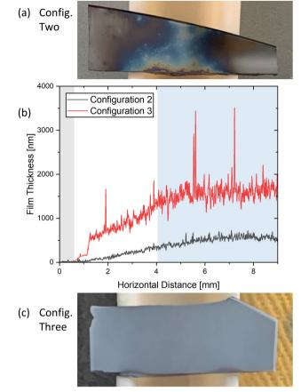
Fig. 3 (a) Photograph of SiO<sub>2</sub> deposition by PVD configuration two i.e., alumina boat without quartz tube. (b) SiO<sub>2</sub> film thickness measurements across samples (a) and (c). (c) Photograph of SiO<sub>2</sub> deposition by configuration three i.e., the alumina boat contained within a hollow guartz tube configuration. Both depositions were carried out under the same conditions (~47.5 mg PDMS, 650 °C steady-state deposition temperature, 12 °C min<sup>-1</sup> heating rate).
