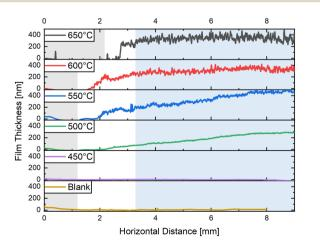
Fig. 6 Steady-state deposition temperature dependence of SiO<sub>2</sub> film thickness using 12 mg of PDMS at a heating rate of 12 °C minute<sup>-1</sup>.
