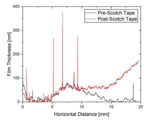
Fig. 7 SiO<sub>2</sub> coating without Si piece to mark uncoated areas alongside a scan across the same sample after the "Scotch-Tape" test performed on the latter half of the surface (10-20 mm)
