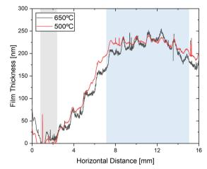
Fig. 9 SiO<sub>2</sub> coating at steady-state deposition temperatures of 500 °C and 650 °C, each using 1.5 mg of PDMS and a heating rate of 12 °C minute<sup>-1</sup>.
