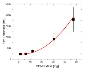
Fig. 5 Film thickness vs. PDMS mass using a 12 °C min<sup>-1</sup> heat rate, and a steady-state deposition temperature of 650 °C. The red line is a guide to the eye, using a parabolic form with a constant offset.
