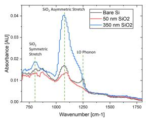
Fig. 13 (a) FTIR spectra of the SiO<sub>2</sub> coatings at varying thicknesses, showing the symmetric and asymmetric stretching vibrations of Si-O-Si at 800 and 1100 cm<sup>-1</sup> respectively, and longitudinal optical phonons of the crystalline silicon wafer and its native oxide at 1250 cm<sup>-1</sup> in the uncoated substrate
