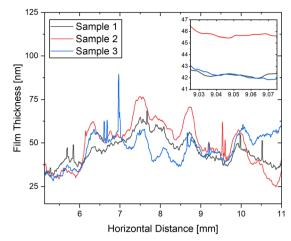
Fig. 11 Profilometry scans of three different substrates subjected to SiO<sub>2</sub> PVD using 6 mg PDMS and 1 °C minute<sup>-1</sup> heat rates using a steady-state deposition temperature of 500 °C, demonstrating the process reproducibility for deposition of very thin films across a large area along the centre of the alumina boat. (Inset; Higher magnification view of the SiO<sub>2</sub> thickness across a 50 µm long region on the sample).
