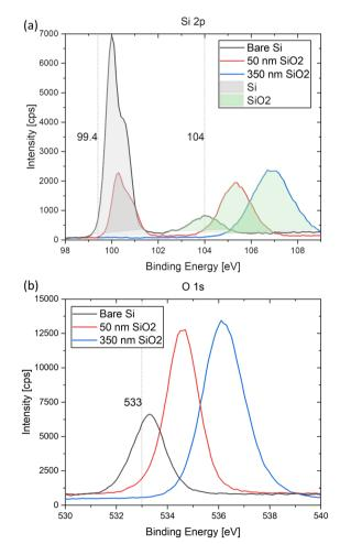
Fig. 14 XPS spectra of SiO<sub>2</sub> coatings of varying thicknesses of the (a) Si 2p region showing the decrease in Si signal (99.4 eV) and increasing oxide signal (104+ eV) with increasing SiO<sub>2</sub> thickness, and the (b) O 1s region showing the increasing O signal ( $\sim$  533 eV) with increasing SiO<sub>2</sub> thickness. Both spectra show surface charging effects.
