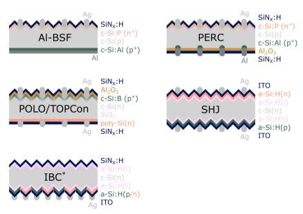
Fig. 1 Schematic illustration of different single junction crystalline silicon cell architectures. \*The IBC structure is depicted with a-Si passivation, however, multiple different approaches are possible.
