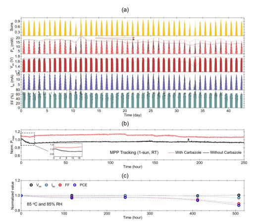
Fig. 14 Outdoor testing results over 43 days for perovskite/silicon tandem cell. (a) Light intensity, power output, V<sub>OC</sub>, I<sub>SC</sub> and FF, (b) power output of cells under constant illumination for 250 hours, (c) damp heat testing at 85 °C at 85% RH. 146
