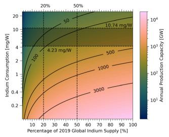
Fig. 13 Calculated allowable annual production capacity for SHJ solar cells as a function of both the indium consumption (mg  $W^{-1}$ ) per cell and % of 2019 global indium supply. 136
