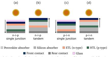
Fig. 5 (a) n-i-p perovskite single junction solar cell where the n-type contact faces the sun, (b) n-i-p perovskite/silicon tandem solar cell where the ptype contact faces the sun, (c) p-i-n perovskite single junction solar cell where the p-type contact faces the sun, (d) p-i-n perovskite/silicon tandem solar cell where the n-type contact faces the sun
