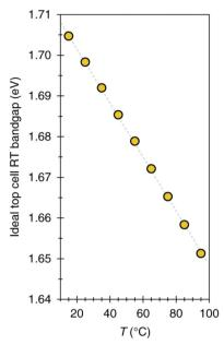
Fig. 15 Calculated optimum perovskite  $E_{\rm g}$  for maximising efficiency under AM1.5 irradiance under varied operating temperature. 149
