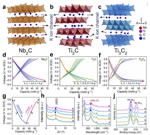
Fig. 8 Crystal structures of (a)  $Nb_2C$ , (b)  $Ti_2C$ , and (c)  $Ti_3C_2$ . GCD profiles at different rates for (d)  $Nb_2C$ , (e)  $Ti_2C$ , and (f)  $Ti_3C_2$ . (g) GCD curves of  $Nb_2C$  cathode at 0.5 A g<sup>-1</sup>. The corresponding (h) XRD, (i) Raman, and (j) XPS data during the cycling. Reproduced with permission from ref. 55. Copyright 2022, Tsinghua University Press.
