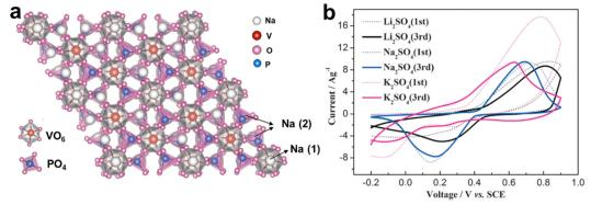
Fig. 6 (a) Crystal structure of Na<sub>3</sub>V<sub>2</sub>(PO<sub>4</sub>)<sub>3</sub>. (b) CV curves of Na<sub>3</sub>V<sub>2</sub>(PO<sub>4</sub>)<sub>3</sub> at 5 mV s<sup>-1</sup> in 1 M K<sub>2</sub>SO<sub>4</sub>, Na<sub>2</sub>SO<sub>4</sub>, and Li<sub>2</sub>SO<sub>4</sub> electrolytes. Reproduced with permission from ref. 51. Copyright 2014, Wiley-VCH.
