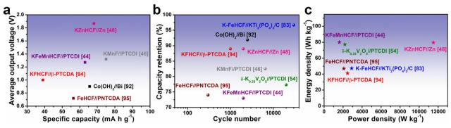
Fig. 16 (a) Average output voltage versus specific capacity, (b) capacity retention versus cycle number, and (c) energy density versus power density of selected AKIB full cells reported in the literature.
