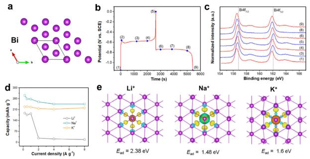
Fig. 11 (a) Crystal structure of Bi. (b) The second GCD profiles of Bi anode at 1 mA cm<sup>-2</sup>. (c) Corresponding ex situ XPS spectrum. Reproduced with permission from ref. 92. Copyright 2020, Elsevier Inc. (d) Rate performance of Bi anode in K+/Na+/Li+ electrolytes. (e) The charge density difference induced by three ions absorption, respectively. Reproduced with permission from ref. 93. Copyright 2022, Elsevier Inc.
