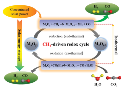
Fig. 1 Schematic of two-step solar thermochemical carbon dioxide splitting and water splitting processes coupled with methane driven reduction (MDR-STCDS, MDR-STWS).
