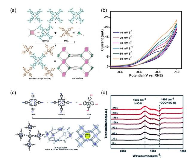
Fig. 25 (a) Synthesis of MPc-PI-COF-3 ( $M = Co^{II}$  or  $H_2$ ) and (b) scan rate dependence of cyclic voltammetry response of CoPc-PI-COF-3. (c) Schematic representation of the synthesis of 3D-Por(Co/H)-COF and the simulated network. (d) In situ ATR-IR of 3D-Por(Co/H)-COF at -0.9 V. (a and b) Reproduced with permission.<sup>274</sup> Copyright 2022, John Wiley and Sons Ltd. (c and d) Reproduced with permission.<sup>275</sup> Copyright 2022, Royal Society of Chemistry.
