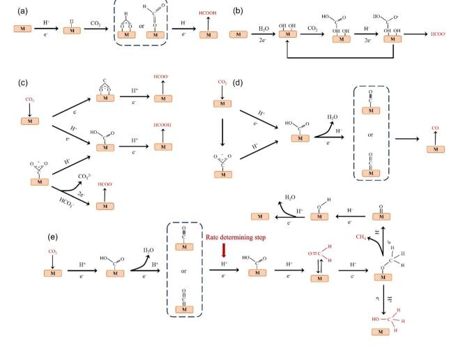
Fig. 3 (a) Monodentate or bidentate intermediate route for HCOOH formation. (b) Surface-bound carbonate intermediate route for the formation of HCOOH/formate. (c)  $*CO_2$  radical intermediate route for the formation of formate. (d) Possible reaction pathway of  $CO_2$  reduction to CO. (e) Possible reaction pathways for the reduction of  $CO_2$  to HCHO,  $CH_3OH$  and  $CH_4$ .
