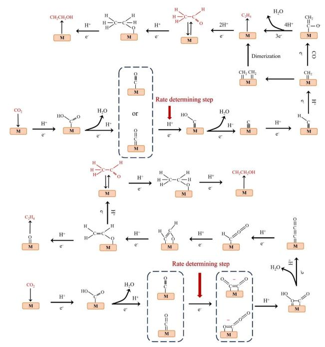
Fig. 4 Possible reaction paths for electrocatalytic  $CO_2$  reduction to produce  $C_2H_4$ ,  $CH_3CHO$ , and  $C_2H_5OH$ .
