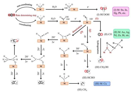
Fig. 2 Schematic mechanism of various metal electrocatalysts for the CO<sub>2</sub>RR.
