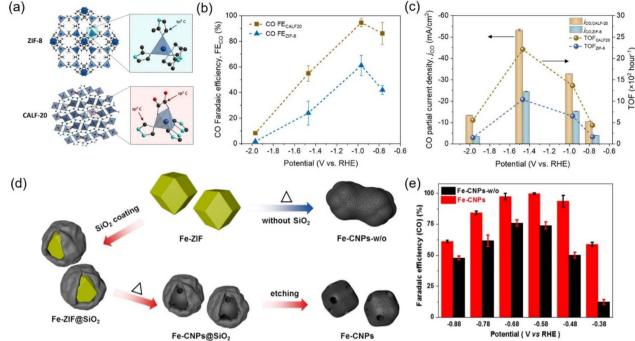
Fig. 22 (a) Schematic illustration of the crystal structure of ZIF-8 and CALF20. (b) FE<sub>CO</sub> and (c) CO partial current densities and TOF at different applied potentials for CALF20 and ZIF-8 in 1.0 M KOH. (d) Synthetic illustration of Fe-CNPs and Fe-CNPs-w/o. (e) FE<sub>CO</sub> at different potentials. (ac) Reproduced with permission.<sup>249</sup> Copyright 2021, American Chemical Society. (d and e) Reproduced with permission.<sup>252</sup> Copyright 2019, American Chemical Society
