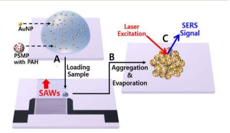
Fig. 1 Schematic representation of detecting polycyclic aromatic hydrocarbons (PAHs) adsorbed on polystyrene microparticles (PSMPs) using surfaced-enhanced Raman spectroscopy (SERS) based on surface acoustic waves (SAWs). (A) A 1 μL droplet consisting of 1 μm PSMPs and 50 nm gold nanoparticles (AuNPs) is loaded on the SAW chip. (B) After being aggregated and evaporated completely by the SAWs, (C) SERS signals are measured from the cluster with 785 nm laser excitation on 1 mW for 1 s.
