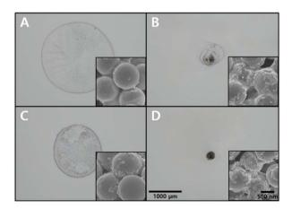
Fig. 3 Microscopic and SEM images of aggregated 50 nm AuNPs mixed with 1  $\mu m$  PSMPs adsorbed with pyrene depending on various conditions: (A) on the original LiNbO $_3$  surface without SAWs, (B) on the original LiNbO $_3$  surface with SAWs, (C) on the hydrophobic coated LiNbO $_3$  surface without SAWs, (D) on the hydrophobic coated LiNbO $_3$  surface with SAWs. Each 1  $\mu L$  of the droplet was loaded on the LiNbO $_3$  surface.
