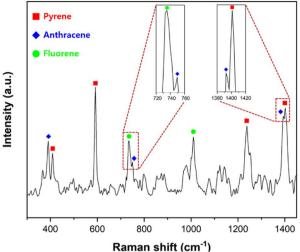
Fig. 7 SERS spectrum of a mixture of 3 PAHs (pyrene, anthracene, fluorene) with a total concentration of 10 mM adsorbed on 1  $\mu$ m PSMPs. Discriminant peaks of each PAH are labeled with different symbols. Peaks with similar shifts are partially overlapped and observed as broad peaks.
