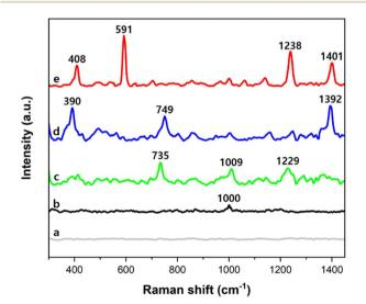
Fig. 5 (a) Raman spectrum measured from the cluster of 1  $\mu$ m PSMPs without AuNPs. SERS spectra measured from the clusters of 50 nm AuNPs and 1  $\mu$ m PSMPs, which adsorbed (b) no PAHs, (c) fluorene, (d) anthracene, and (e) pyrene. 10 mM PAH solution was used for the PSMPs to adsorb a PAH, respectively. Detected SERS characteristic peaks of each PAH are comparable with their own Raman characteristic peaks.
