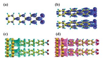
Fig. 7 The local density of states (LDOS) of the LUMO for the isolated  $Pyr|3P|NO_2$  molecule (a), and of the LUPS of the  $Au|Pyr|3P|NO_2$  combined system (b). (c), (d) A 3D isodensity representation of charge rearrangement for  $Au|Pyr|3P|NO_2$  (only the top two layers of the Au-slab are shown). Electrons flow from regions shown in (c) to those depicted in (d).
