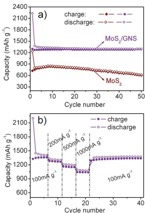
**Fig. 3** (a) Cycling behaviors of MoS<sub>2</sub> and MoS<sub>2</sub>/GNS at a current density of 100 mA g<sup>-1</sup>. (b) Cycling behavior of MoS<sub>2</sub>/GNS at various current densities.
