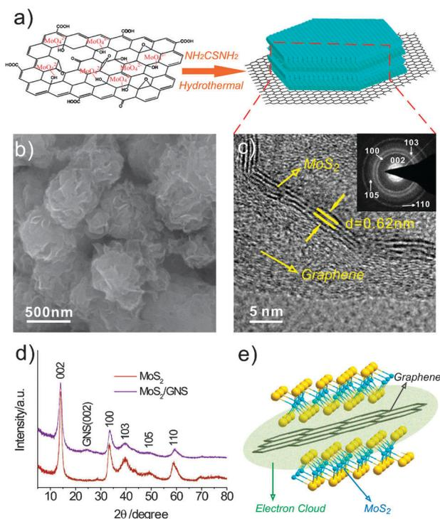
**Fig. 1** (a) Schematic diagram of the *in situ* synthesis of MoS<sub>2</sub>/GNS. (b) SEM image of MoS<sub>2</sub>/GNS composites. (c) HRTEM image of MoS<sub>2</sub> layers on graphene. (d) XRD patterns of MoS<sub>2</sub> and MoS<sub>2</sub>/GNS; inset shows the electron diffraction pattern of the MoS<sub>2</sub> nanosheets on graphene. (e) Schematic illustration of the microstructure of MoS<sub>2</sub>/GNS.
