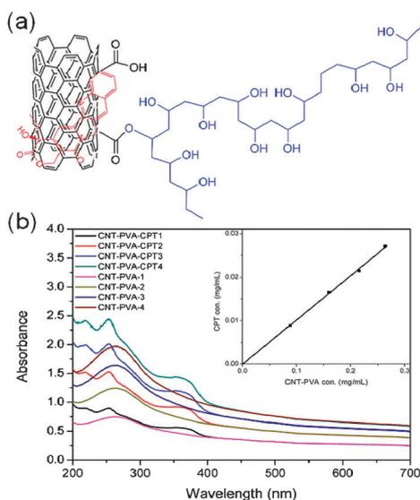
**Fig. 2** CPT loading on MWCNT-PVA: (a) schematic depiction of CPT loaded MWCNT-PVA, and (b) UV spectra of MWCNT-PVA and MWCNT-PVA-CPT with different concentrations.
