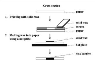
Fig. 1 Schematic diagram of the fabrication step for wax screen-printing method.
