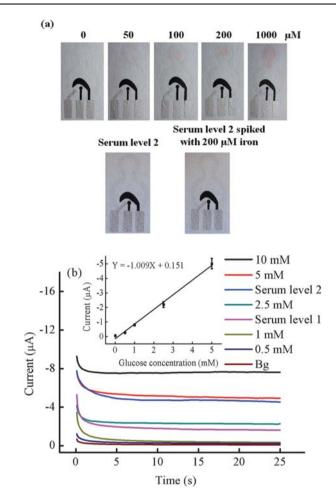
Fig. 5 (a) Photographs of the result for the total iron analysis using colorimetric method. (b) Chronoamperograms of glucose (0-10 mM) determination at -0.2 V versus an on-chip Ag/AgCl. The calibration plot of anodic currents at 20 s of sampling time for determination of three analytes are shown in the inset, n = 3.
