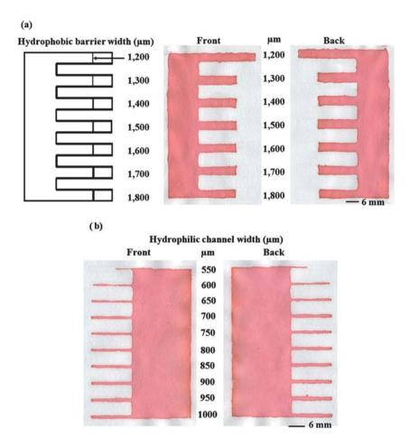
Fig. 3 Resolution of the wax screen-printing method showing (a) the smallest hydrophobic barrier width and (b) the smallest hydrophilic channel width.
