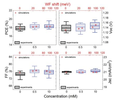
Fig. 4 PCE,  $V_{\text{oc}}$ , FF and  $J_{\text{sc}}$  of n-i-p devices with structure FTO/TiO<sub>2</sub> (compact and mesoporous)/perovskite/csc5/spiro-OMeTAD/Au for different values of negative WF shift. The box charts are the values obtained experimentally from J-V curves measured at 0.01 V s<sup>-1</sup>, while the red circles represent how the PV parameters change depending on the WF shift according to drift-diffusion simulations
