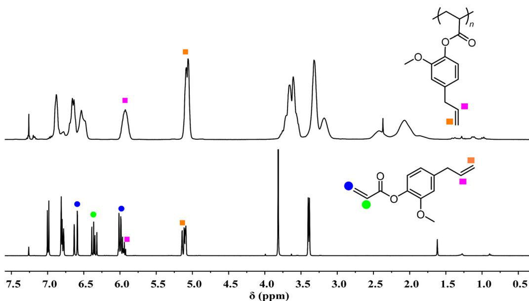
Fig. 4  $^1\text{H}$  NMR spectra ( $\text{CDCl}_3$ , RT): (top) P4aGA produced by the  $\text{DP}^t\text{Bu}_2/\text{B}(2,4\text{-F}_2\text{C}_6\text{H}_3)_3$  FLP (Table 1, run 13); (bottom) 4aGA monomer.
