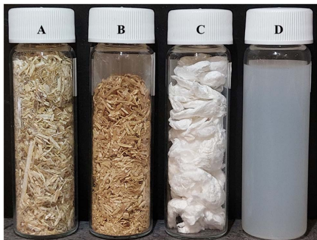
Fig. 2 Photograph of (A) RH, (B) AH, (C) BH and (D) acid hydrolyzed suspension Hemp fibers.
