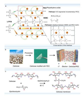
Fig. 8 (a) Schematic illustration of possible Li<sup>+</sup> transport pathways and mechanism in the cellulose//polyethylene oxide (PEO) electrolyte (copyright 2019 The Royal Society of Chemistry); 99 (b) processing from cotton to cellulose and then modified with PEG (copyright 2022 Elsevier B.V.); 100 (c) the cross-linking process of cellulose with epichlorohydrin (copyright 2019 Elsevier B.V.). 101
