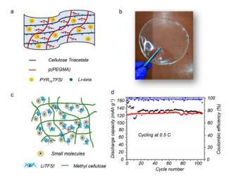
Fig. 11 (a) Available sites for Li coordination and (b) photograph of the cellulose-based solid electrolyte with an ionic liquid (PYR<sub>14</sub>TFSI) (copyright 2021 American Chemical Society); 122 (c) the methyl cellulose-based electrolyte with small molecules (copyright 2020 American Chemical Society); 123 (d) cycling performance at 0.5C of the solid LiFePO<sub>4</sub>//Li cell (copyright 2020 American Chemical Society). 123
