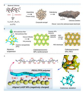
Fig. 9 (a) Schematic illustration of the fabrication of the multifunctional cellulose/LLZTO solid composite electrolyte (copyright 2022 Elsevier B.V.);<sup>111</sup> (b) schematic illustration of fabrication processes for the cellulose/ceramic/PEO solid electrolyte (copyright 2020 American Chemical Society); 112 (c) schematic illustration of the proposed Li+ conducting mechanism in the cellulose/ceramic/PEO solid electrolyte (copyright 2020 American Chemical Society). 112
