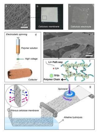
Fig. 4 (a) SEM image and photographs of cellulosic membranes (b) before and (c) after immersion in the electrolyte (copyright 2016 Springer);81 (d) schematic diagram of electrospinning; (e) SEM image and (f) schematic illustration of Li-ion transport of cellulosic membranes (copyright 2024 Springer);82 (g) schematic representation of mass production of a fibrous cellulose membrane using the forcespinning technique (copyright 2015 Springer).83
