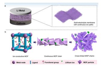
Fig. 10 (a) Schematic illustration of the solid electrolyte of the crosslinked MOF grown on bacterial cellulose; 118 (b) bottom-up synthesis of cross-linked MOF chains on a bacterial cellulose skeleton. (copyright 2021 American Chemical Society). 118
