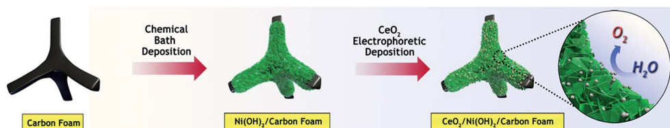
Fig. 1 Process for the design of a self-supported CeO 2 /Ni(OH) 2 /NOSCF electrode and application for the oxygen evolution reaction.
