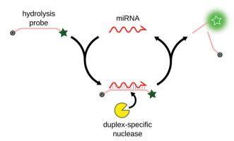
Fig. 7 Principle of DSNSA. Hybridization of the miRNA to a complementary DNA hydrolysis probe forms a RNA/DNA duplex. The duplex-specific nuclease recognizes the duplex and selectively degrades the probe, producing fluorescence. The miRNA remains untouched and is free to bind to another hydrolysis probe, triggering its degradation.
