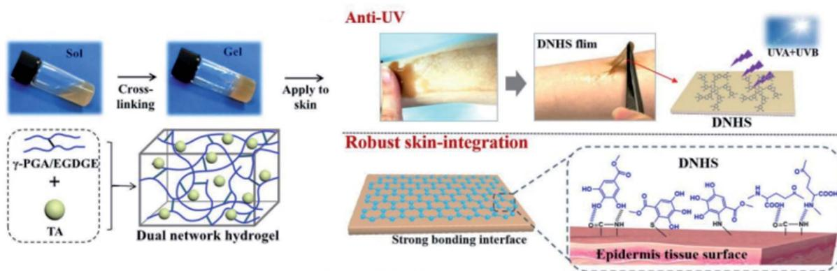
Fig. 16 Chemical crosslinking structure of a dual-network hydrogel sunscreen (DNHS) and its skin adhesion mechanism. Reproduced from ref. 147 with permission from the American Chemical Society, copyright 2019.
