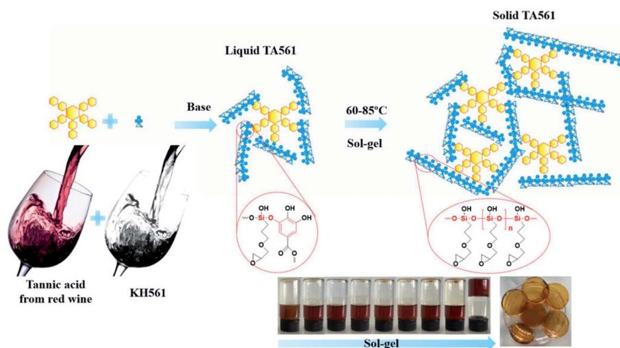
Fig. 10 Synthetic production of TA-KH561 copolymer under mild conditions. Reproduced from ref. 109 with permission from the Royal Society of Chemistry, copyright 2021.
