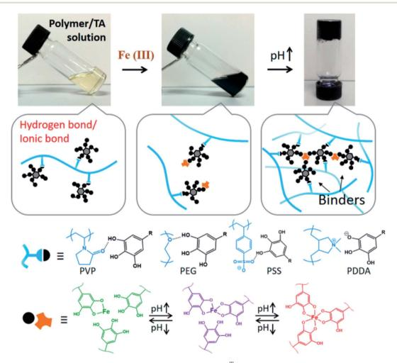
Fig. 5 Formation mechanism of TA-polymer hydrogels based on polymer/TA/Fe<sup>III</sup>. Reproduced from ref. 68 with permission from the American Chemical Society, copyright 2017.
