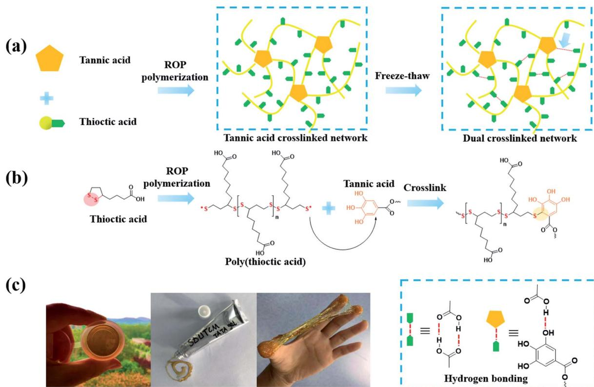
Fig. 14 (a) A schematic illustration of the synthetic route of TATA hydrogel; (b) Mechanism of the polyphenol–thiyl radical oxidation reaction; (c) photos of the TATA hydrogel. Reproduced from ref. 131 with permission from the Royal Society of Chemistry, copyright 2021.
