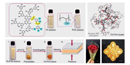
Fig. 2 Schematic illustration of the preparation process of TA-PVA composites. Reproduced from ref. 41 with permission from the American Chemical Society, copyright 2020.
