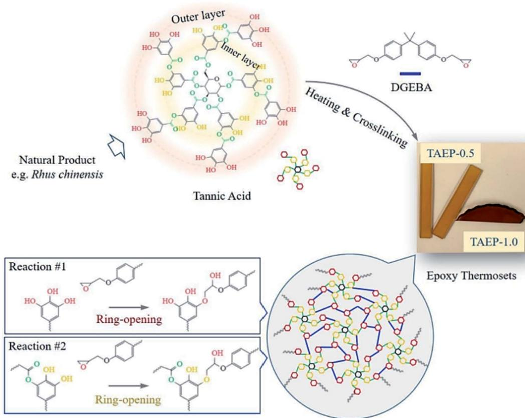
Fig. 9 The polymerization between TA and epoxy monomer (DGEBA) to produce tunable thermosets. Reproduced from ref. 103 with permission from the American Chemical Society, copyright 2020.
