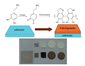
Scheme 1 Multifunctional coating formation by oxidant-induced dopamine polymerization (left to right: glass, Al, polyethersulfone, nylon and cellulose).
