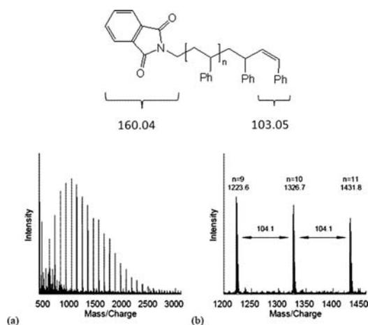
**Fig. 3** ES<sup>+</sup> MS of polystyrene after end group removal *via* thermolysis,  $1326.7 = (10 \times 104.06) + 160.04 + 103.05 + 22.99 (\text{Na}^+)$ , the interpeak distance corresponding to the mass of the styrene repeat unit (104.1).<sup>55</sup>
