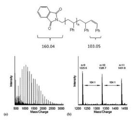
Fig. 3 ES<sup>+</sup> MS of polystyrene after end group removal *via* thermolysis,  $1326.7 = (10 \times 104.06) + 160.04 + 103.05 + 22.99$  (Na<sup>+</sup>), the interpeak distance corresponding to the mass of the styrene repeat unit (104.1).<sup>55</sup>
