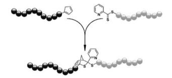
Scheme 12 General synthetic strategy for producing well-defined high  $M_w$  block copolymers via the RAFT-HDA click reaction (TFA, CHCl<sub>3</sub>, RT).<sup>84</sup>
