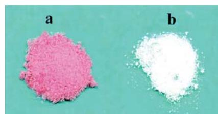
**Fig. 2** Picture of poly(methyl methacrylate) (PMMA) synthesised by the RAFT process (a) before and (b) after reaction with AIBN.<sup>45</sup>
