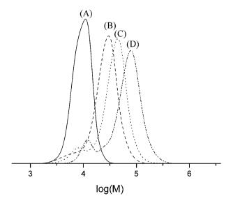
**Fig. 6** SEC traces of (A) P(BLG-co-FMOCLLys), (B) P(BLG<sub>40</sub>-co-(Lys<sub>10</sub>-g-PBLG<sub>20</sub>), (C) P(BLG<sub>40</sub>-co-(Lys<sub>10</sub>-g-PBLG<sub>20</sub>) and (D) P(BLG<sub>40</sub>-co-(Lys<sub>10</sub>-g-PBLG<sub>40</sub>) measured by DMF-SEC calibrated with polystyrene standards. Subscript numbers denote the targeted degree of polymerization.
