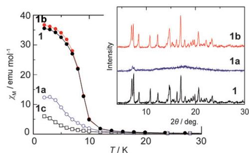
**Fig. 3** Temperature dependences of  $\chi_M$  for the initial form **1** (●), the dehydrated form **1a** (○), the rehydrated form **1b** (●) and the anhydrous form **1c** (□) in an applied dc field of 500 Oe. The insert shows the corresponding XRPD patterns.
