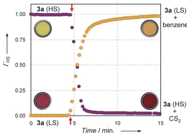
**Fig. 9** Time dependence of the fraction of the HS state under a benzene (yellow) and  $\text{CS}_2$  (purple) atmosphere at 293 K. Red arrows indicate the starting points of guest injection (valve opening). The color circles are photos of samples.
