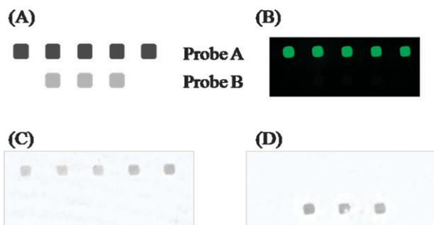
**Fig. 3** (A) The slide glass was spotted with PNA probes A and B. (B) Fluorescent images of DNA chips with a 10 nM Cy3-labeled target A. (C) Optical scanner image of a 10 nM target A (18-mer) hybridized DNA chip. The intensity of the grayscale value was *ca.* 49. (D) Scanner image of a 10 nM target B (50-mer) hybridized DNA chip, showing a stronger response, with a grayscale value of *ca.* 64.
