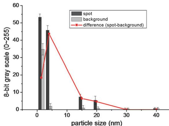
**Fig. 2** Comparison of the grayscale response for various gold nanoparticle sizes (1.4, 4, 15, 20, 30, and 40 nm). The optimal particle size was 4 nm, resulting in the highest net difference between the spot and background.
