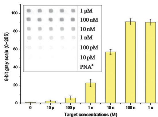
**Fig. 4** Graph of 8-bit grayscale values depending on the concentration of target A. The concentrations of target DNA, from bottom to top, were 0, 0.01, 0.1, 1, 10, 100, and 1000 nM. The gray level increased with increasing target concentration. Inset: optical scanner images of different target concentrations. (\*Only PNA probe without hybridization).
