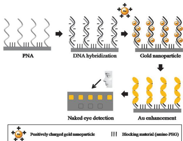
**Fig. 1** Schematic diagram of DNA detection strategy by the naked eye or an optical scanner.
