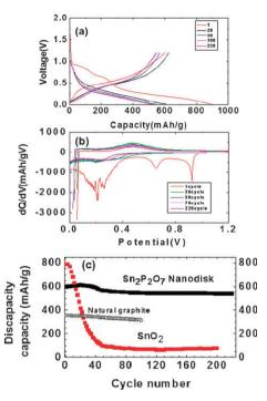
**Fig. 2** (a) Voltage profiles of the quenched nanodisks in a coin-type half cell between 0 and 1.2 V at 0.5 C rate (= 350 mA g<sup>-1</sup>) after 1, 20, 50, 100, 220 cycles. (b) Differential curves of (a). (c) Discharge capacity (after lithium removal) *vs.* cycle number in nanodisk. References are natural graphite and SnO<sub>2</sub> nanoparticles.
