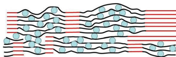
**Fig. 6** Cross-sectional schematic drawing (not to scale) of a high-capacity, stable electrode, made of a continuous, conducting 3-D network of graphite (red) anchoring regions of graphene–Si composite. Blue circles: Si nanoparticles, black lines: graphene sheets.
