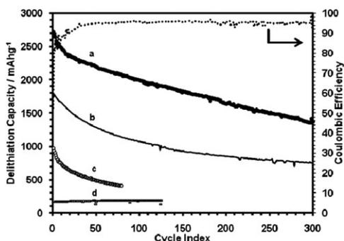
**Fig. 5** Delithiation capacity of: (a) SG paper sample 2, 61 wt% Si, shown with coulombic efficiencies; (b) SG paper sample 1, 59 wt% Si, tested using the CCCV method (sample 1: 1.5–0.005 V, 1000–80 mA g<sup>-1</sup>; sample 2: 1.5–0.02 V, 1000–50 mA g<sup>-1</sup>); (c) SG paper sample 1, crushed and mixed with PVDF binder, cycled at 100 mA g<sup>-1</sup> constant current mode (2.0–0.02 V); (d) graphene-only sample cycled using CCCV method.
