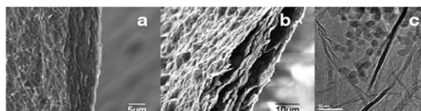
**Fig. 3** Edge-view SEM images of: (a) SGO paper; (b) SG paper, and TEM images of: (c) SG paper.
