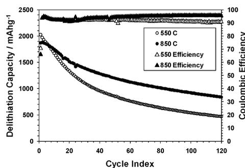
**Fig. 4** Delithiation capacities and coulomb efficiencies of SG samples reduced at 550 or  $850^\circ\text{C}$ , using a constant current–constant voltage (CCCV) method ( $1.5\text{--}0.020 \text{ V}$ ,  $1000\text{--}50 \text{ mA g}^{-1}$ ).
