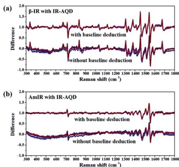
Fig. 2 Mid-frequency Raman difference spectra (MFRDS) with and without baseline deduction of (a)  $\beta$ -IR and (b) AmIR with IR-AQD. MFRDS with baseline deduction are shown with a translation on the vertical axis for clear. Each sample was characterized three times individually, and the corresponding nine MFRDS are shown here.
