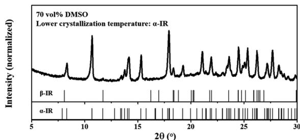
Fig. 4 PXRD pattern of the recrystallized product from saturated 70 vol% DMSO solution of IR (the solution was cooled from 60 °C to –18 °C).  $\beta$ -IR was prepared by cooling the solution from 60 °C to room temperature.
