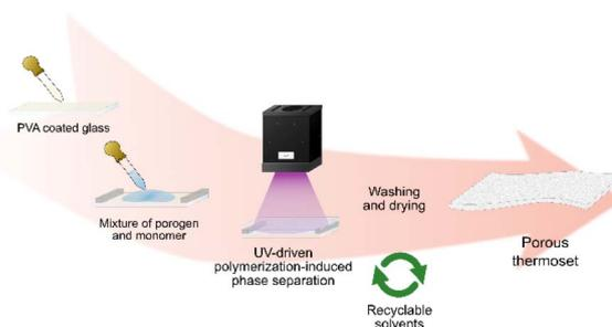
Fig. 2 Process schematic of thermoset membrane fabrication.
