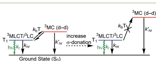
Fig. 1 Partial excited-state diagram for cyclometalated iridium complexes, showing partial occupation of  $^3\text{MC}$  states and destabilization of these states when stronger  $\sigma$ -donor ligands are incorporated.
