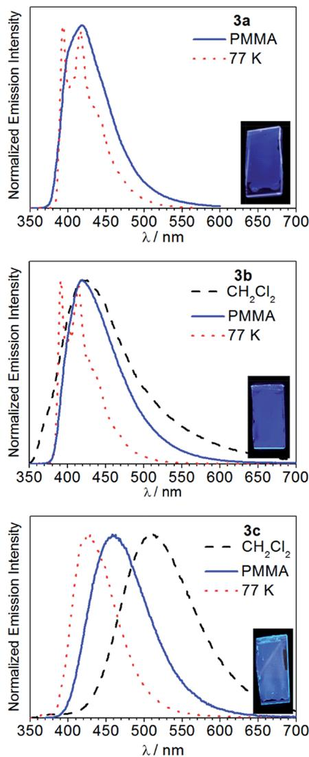
Fig. 5 Photoluminescence spectra of **3a–c** recorded in  $\text{CH}_2\text{Cl}_2$  at room temperature (black trace, dashed line), PMMA film at room temperature (blue trace, solid line), and in 1 : 3  $\text{CH}_2\text{Cl}_2$ /toluene glass at 77 K (red trace, dotted line). Samples were excited at  $\lambda = 310$  nm. The insets show photographs of the PMMA films under UV illumination.
