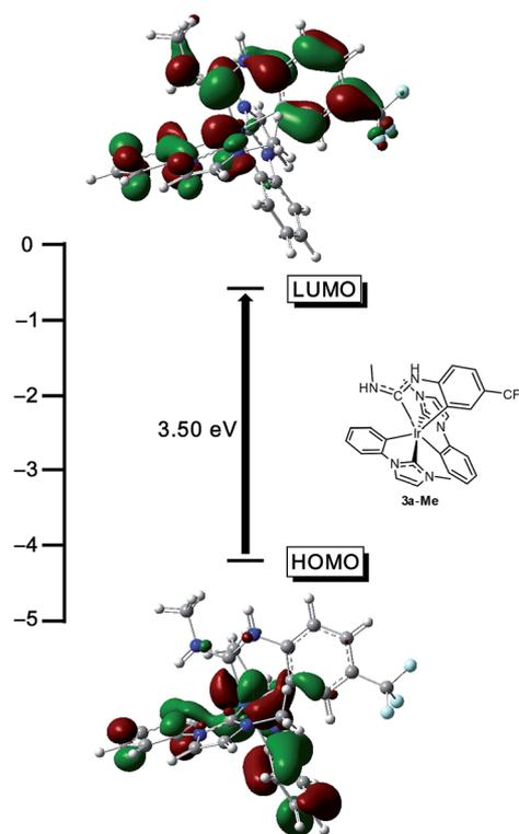
Fig. 7 DFT-computed HOMO and LUMO energy values and plots for the model complex **3a-Me** (isovalue = 0.03 a.u.). Calculations were performed in the gas phase at MN15L/6-311G\* for nonmetal atoms, with the SDD basis set used for Ir. The structure of **3a-Me** is also shown, in the approximate orientation used for the orbital depictions.
