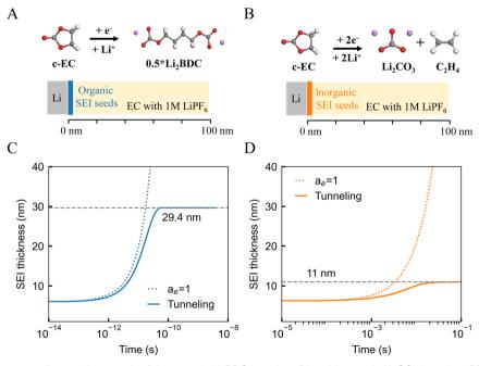
Fig. 3 The effect of electron tunneling on the growth of the organic Li<sub>2</sub>BDC based on R1 and inorganic Li<sub>2</sub>CO<sub>3</sub> based on R3. (A) and (B) Illustrations of reactions R1 and R3 considered and the 1D system, respectively, (C) comparison of organic  $Li_2BDC$  growth behaviors between assuming  $a_{e^-} = 1$  and electron tunneling, and (D) comparison of inorganic  $Li_2CO_3$  growth behaviors assuming  $a_{e^-} = 1$  and electron tunneling
