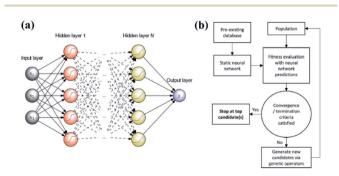
Fig. 7 (a) An example of a feed-forward ANN with N hidden layers and a single neuron in the output layer.<sup>80</sup> (b) Schematic of an ANN-evaluated genetic algorithm.<sup>74</sup>
