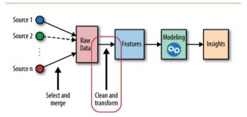
Fig. 1 The machine learning workflow; the place of feature engineering is shown in the red circle.  $^{11}$
