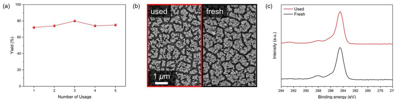
Fig. 4 Stability test for iterative usage of the photoanode. (a) Yield of the reaction under the “standard conditions” for five iterative uses. (b) SEM image of a hematite photoanode before and after five iterative uses under the standard reaction conditions. (c) XPS spectra of carbon 1s region before and after five iterative uses.
