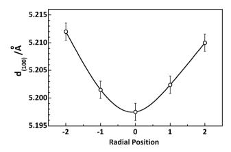
Fig. 7 Variety of d-spacing at different radial positions in PAN filament.
