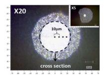
Fig. 2 Schematic of the cross-section scanning of PAN fibre by micro-Raman spectra.
