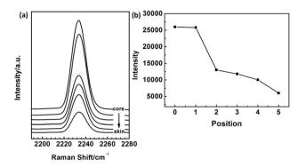
Fig. 15 The intensity of  $v_{\rm CN}$  peak in Raman spectra for PAN fiber with different radial position.
