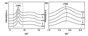
Fig. 5 (a) WAXD profiles and (b) (100) diffraction peak of PAN fibres acquired in different radial positions.
