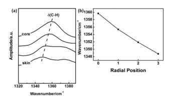
Fig. 14 The peak shift of IR absorption  $\delta(\text{C-H})$  with different radial position in PAN filament.
