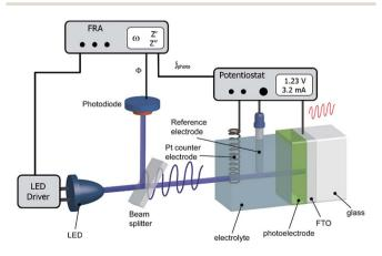
Fig. 1 Schematic diagram of the intensity modulated photocurrent spectroscopy (IMPS) setup. Modulated illumination is provided by a light emitting diode ( $\lambda = 455$  nm), and the modulated photocurrent response of the sample is measured and analyzed.
