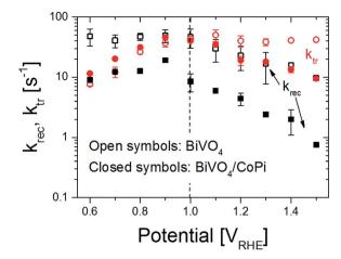
Fig. 4 Charge transfer rate constant (red) and recombination rate constant (black) for the unmodified (open symbols) and the CoPi modified  ${\rm BiVO_4}$  (closed symbols). The error bars represent the spread in the results obtained for different samples at selected potentials; in total, three bare  ${\rm BiVO_4}$  electrodes and two  ${\rm BiVO_4/CoPi}$  electrodes were measured.
