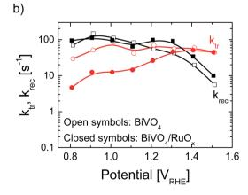
Fig. 5 (a) Photocurrent–voltage (j-V) curve of bare BiVO<sub>4</sub> (black) and RuO<sub>x</sub> modified BiVO<sub>4</sub> (red) taken under illumination with a 455 nm LED  $(\varphi=4~{\rm mW~cm^{-2}})$ . (b) Charge transfer rate (red) and recombination rate constant (black) for the unmodified (open symbols) and the RuO<sub>x</sub> modified BiVO<sub>4</sub> (closed symbols).
