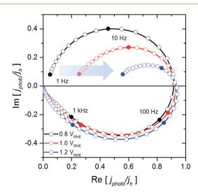
Fig. 2 IMPS spectra of BiVO<sub>4</sub> photoanode under different applied potentials. The increase of low-frequency intercepts with increasing potential, indicate an improvement of the charge transfer efficiency.
