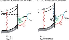
Fig. 6 Simplified model of the elementary processes in a BiVO<sub>4</sub> photoanode (a) without a co-catalyst (b) with a surface passivating co-catalyst (e.g. CoPi) and (c) with a non-passivating co-catalyst (e.g.  $RuO_x$ ). Upon illumination, photo-excited carriers move towards the semiconductor–electrolyte interface, where direct water oxidation by valence band holes (1), surface state–mediated recombination (2), and charge transfer via co-catalyst (3) can take place.
