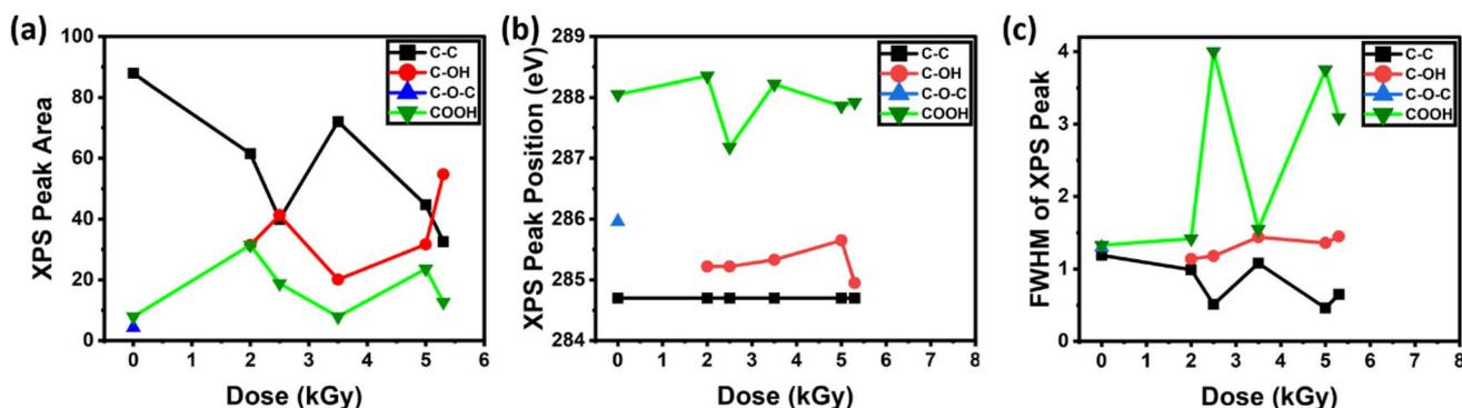
Fig. 5 (a) XPS peak area as a function of irradiation dose. (b) XPS peak position as a function of irradiation dose. (c) Full width at half maximum (FWHM) of XPS peaks as a function of irradiation dose.
