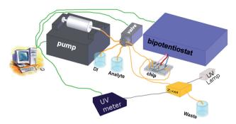
Fig. 4 Setup used in the cyclic voltammetry and conversion efficiency measurements.
