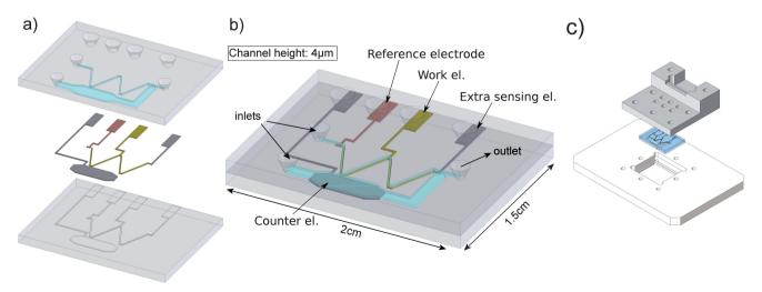
Fig. 3 Overview of the fabricated chip. a) Bottom layer with recess etched wells for the electrodes and top wafer with inlets and fluidic channels. b) Assembled view of the total chip (1.5 by 2 cm) and the different electrodes and inlets indicated. c) Chip and chipholder.
