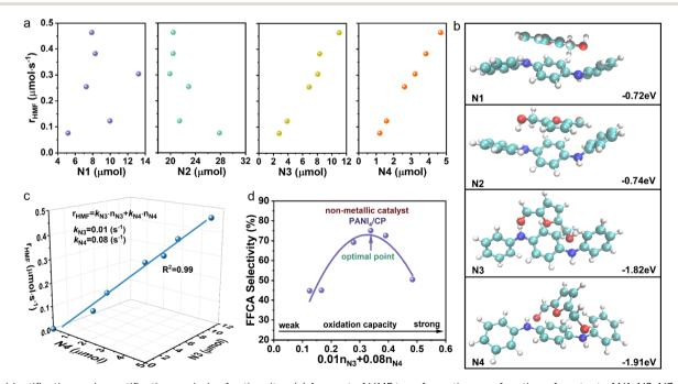
Fig. 4 Identification and quantification analysis of active sites. (a) Amount of HMF transformation as a function of content of N1, N2, N3 and N4, respectively. (b) Optimized structure and adsorption energies of HMF adsorbed on N1, N2, N3 and N4 of PANI, respectively. (c) Content of N3 and N4 as a function of conversion rate of HMF. (d) Contribution of all active sites (oxidation capacity) of PANI catalysts as a function of selectivity of FFCA.
