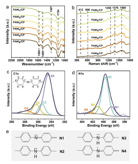
Fig. 2 Chemical structure characterization. (a) FT-IR and (b) Raman spectra of PANI/CP samples. (c) Deconvoluted C 1s XPS and (d) N 1s XPS spectra of PANI<sub>1</sub>/CP samples. (e) Structures of four nitrogen species.
