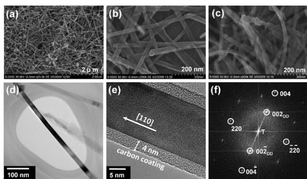
**Fig. 1** Morphological characterization of  $\text{Fe}_3\text{O}_4$  nanowires: (a) low and (b) high magnification FE-SEM images of as-synthesized  $\text{Fe}_3\text{O}_4$  nanowires, (c) FE-SEM image of carbon-decorated  $\text{Fe}_3\text{O}_4$  nanowires, (d) TEM and (e) HRTEM images showing crystalline  $\text{Fe}_3\text{O}_4$  nanowires surrounded by amorphous carbon, and (f) FFT image of single-crystalline  $\text{Fe}_3\text{O}_4$  nanowire. The subscript DD refers to double diffraction.
