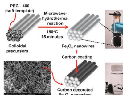
**Scheme 1** Schematic illustration of the microwave-hydrothermal synthesis of single-crystalline Fe<sub>3</sub>O<sub>4</sub> nanowires, employing PEG-400 as a soft template and subsequent carbon decoration for application as high performance anode in lithium ion batteries.
