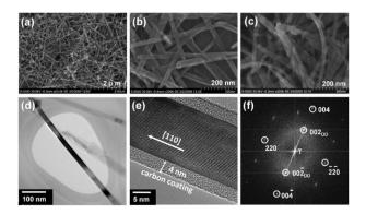
**Fig. 1** Morphological characterization of  $Fe_3O_4$  nanowires: (a) low and (b) high magnification FE-SEM images of as-synthesized  $Fe_3O_4$  nanowires, (c) FE-SEM image of carbon-decorated  $Fe_3O_4$  nanowires, (d) TEM and (e) HRTEM images showing crystalline  $Fe_3O_4$  nanowires surrounded by amorphous carbon, and (f) FFT image of single-crystalline  $Fe_3O_4$  nanowire. The subscript DD refers to double diffraction.
