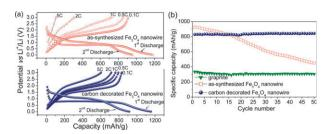
Fig. 3 (a) Galvanostatic charge—discharge curves of as-synthesized and carbon-decorated Fe<sub>3</sub>O<sub>4</sub> nanowires in lithium cells (charged at various C-rates from 0.1C to 5C but discharged at a constant rate of 0.1C) and (b) cycling performances of the Fe<sub>3</sub>O<sub>4</sub> nanowires before and after carbon decoration at 0.1C rate. For a comparison, data for a natural graphite electrode is also shown.
