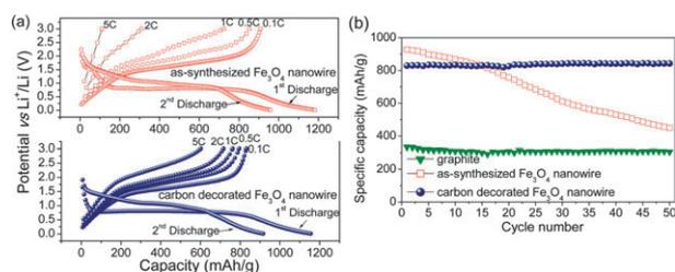
**Fig. 3** (a) Galvanostatic charge–discharge curves of as-synthesized and carbon-decorated  $\text{Fe}_3\text{O}_4$  nanowires in lithium cells (charged at various C-rates from 0.1C to 5C but discharged at a constant rate of 0.1C) and (b) cycling performances of the  $\text{Fe}_3\text{O}_4$  nanowires before and after carbon decoration at 0.1C rate. For a comparison, data for a natural graphite electrode is also shown.
