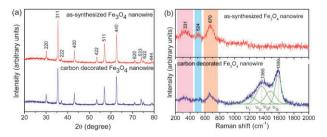
Fig. 2 (a) X-ray diffraction and (b) Raman spectra of  $Fe_3O_4$  nanowires before and after carbon decoration.
