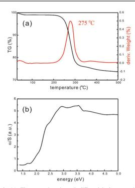
Fig. 3 (a) Thermogravimetric and differential thermogravimetric curves of H-Re/Te/Mn under nitrogen flow (heating rate 10 °C min<sup>-1</sup>). (b) Solid state UV/Vis spectrum of H-Re/Te/Mn. Absorption data were calculated from the reflectance data using the Kubelka-Munk function;  $\alpha/S = (1 - R)^2/2R$ , where R is the reflectance at a given wavenumber,  $\alpha$  is the absorption coefficient, and S is the scattering coefficient. The band gap energy is 1.92 eV.
