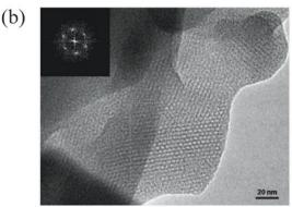
**Fig. 1** (a) Powder XRD patterns of samples prepared at room temperature (L–Re/Te/Mn in black), at 75 °C (HL–Re/Te/Mn in blue); and at 120 °C (H–Re/Te/Mn in red). For the HL–Re/Te/Mn, H- denotes hexagonal phase and L- denotes lamellar phase. (b) TEM image of H–Re/Te/Mn. The inset shows the Fourier-transformed diffraction pattern of the boxed area.
