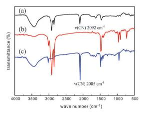
Fig. 2 IR spectrum of compound H-Re/Te/Mn (a), crystalline CTAB (b),  $[(CH_3)_4N]_4[Re_6Te_8(CN)_6]$  (c).
