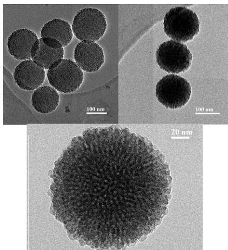
Fig. 1 TEM images of spherical mesoporous silica nanoparticles.
