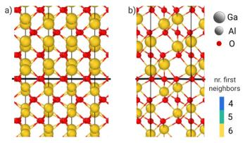
Fig. 3 Front (a) and side (b) view of the  $\alpha$ -Ga<sub>2</sub>O<sub>3</sub>/ $\alpha$ -Al<sub>2</sub>O<sub>3</sub> interface. The black line marks the plane of O atoms shared by both film and substrate.
