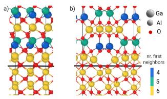
Fig. 5 Front (a) and side (b) view of the  $\kappa$ -Ga<sub>2</sub>O<sub>3</sub>/ $\alpha$ -Al<sub>2</sub>O<sub>3</sub> interface. The black line marks the plane of O atoms shared by both the film and the substrate.
