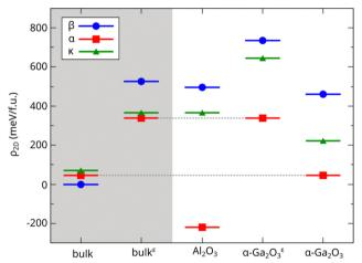
Fig. 7 Diagram of  $\rho_{2D}$  calculated for 2D films of the  $Ga_2O_3$  polymorphs, considering different substrates. The bulk values are reported on the left as a reference, also accounting for the misfit strain induced by the Al<sub>2</sub>O<sub>3</sub> substrate (labelled with  $\varepsilon$ ).
