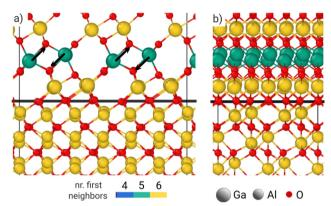
Fig. 4 Front (a) and side (b) view of the  $\beta$ -Ga<sub>2</sub>O<sub>3</sub>/ $\alpha$ -Al<sub>2</sub>O<sub>3</sub> interface. The black line marks the plane of O atoms shared by both film and substrate
