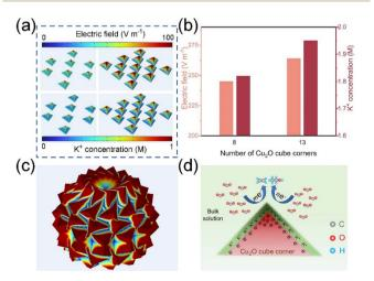
Fig. 1 (a) The electric field (upper half) and K<sup>+</sup> concentration (lower half) distribution on M-4 and M-5 through COMSOL Multiphysics simulations. (b) The electric field and K<sup>+</sup> concentration at the tips of M-4 and M-5. (c) The electric field distribution on M-3. (d) A schematic illustration of the local electric field and K<sup>+</sup> ions on the Cu<sub>2</sub>O cube corner for promoting C<sub>2</sub> formation.
