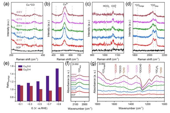
Fig. 4 In situ Raman spectra of the  $Cu_2O-0$  catalyst in the range 200-450 cm<sup>-1</sup> (a), 400-750 cm<sup>-1</sup> (b), 900-1150 cm<sup>-1</sup> (c) and 1800-2200 cm<sup>-1</sup> (d) at various applied potentials (vs. RHE). (e) Ratio of the low-frequency and high-frequency bands in the range 2000-2200 cm<sup>-1</sup> of  $Cu_2O-0$  and  $Cu_2O-4$  catalysts at various applied potentials. (f and g) In situ FT-IR spectra of the  $Cu_2O-0$  catalyst at various applied potentials (vs. RHE).
