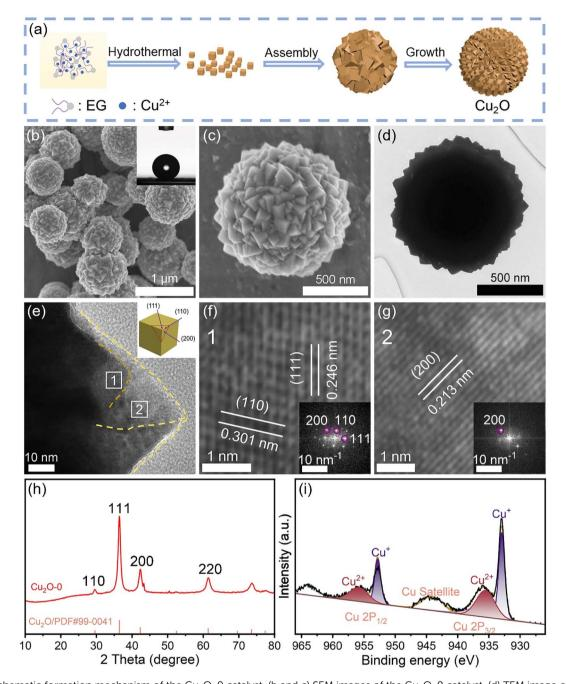
Fig. 2 (a) Schematic formation mechanism of the  $Cu_2O-0$  catalyst. (b and c) SEM images of the  $Cu_2O-0$  catalyst. (d) TEM image of the  $Cu_2O-0$  catalyst. (e-g) HRTEM images of the  $Cu_2O-0$  catalyst. (h) The XRD pattern of the  $Cu_2O-0$  catalyst. (i) The XPS spectrum of the  $Cu_2O-0$  catalyst.
