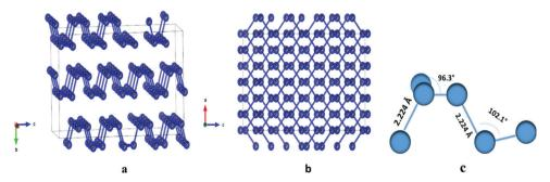
Fig. 1 (a) The crystal structure of BP; (b) crystal structure view along the b-axis; (c) bond length and bond angles of phosphorene.<sup>47</sup>
