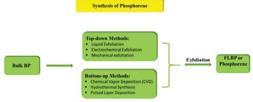
Fig. 2 Different preparative methods of FLBP or phosphorene. 94
