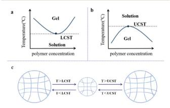
Fig. 3 (a) The LCST-type formulation undergoes sol-gel transition with an increase in temperature. (b) UCST-type formulation undergoes sol-gel transition as the temperature decreases. These figures have been reproduced from ref. 21 with permission from MDPI, copyright 2022. (c) Schematic of the swelling/contraction of the temperature-sensitive hydrogel.
