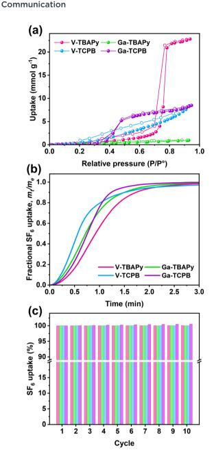
Fig. 3 (a) Water sorption isotherms recorded at 293 K (solid and open spheres represent the adsorption and desorption branches, respectively), (b) gravimetric  $SF_6$  adsorption profiles recorded at 303 K, 100 kPa, and (c) gravimetric  $SF_6$  adsorption cycles.
