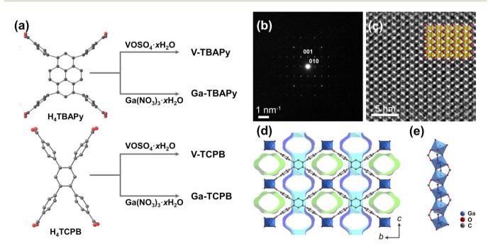
Fig. 1 (a) Synthesis route of Ga- and V-based MOFs with the respective tetratopic  $H_4TBAPy$  and  $H_4TCPB$  ligands, (b) selected area electron diffraction (SAED) image of Ga-TCPB along [100], (c) corresponding HRTEM image with an insert of the crystal structure of Ga-TCPB as viewed along the a-axis, (d) structure of Ga-TCPB as viewed along the a-axis showing the presence of two unique pores (colored in green and blue), and (e) the rod SBU running along the a-axis in the structure.
